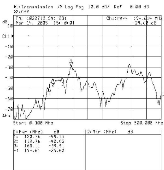
Figure 10: Crosstalk vs frequency in slip ring assemblies
