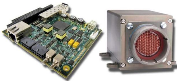
*Figure 20: Two examples of multiplexers are shown. A board level multiplexer that supports multiple uncompressed HD video channels, multiple serial data channels and a single Gigabit Ethernet port. A small Camera Link® multiplexer is shown that converts copper Camera Link signals into a single fiber channel.*
