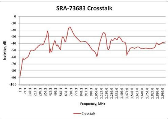
Figure 14: Crosstalk vs frequency
