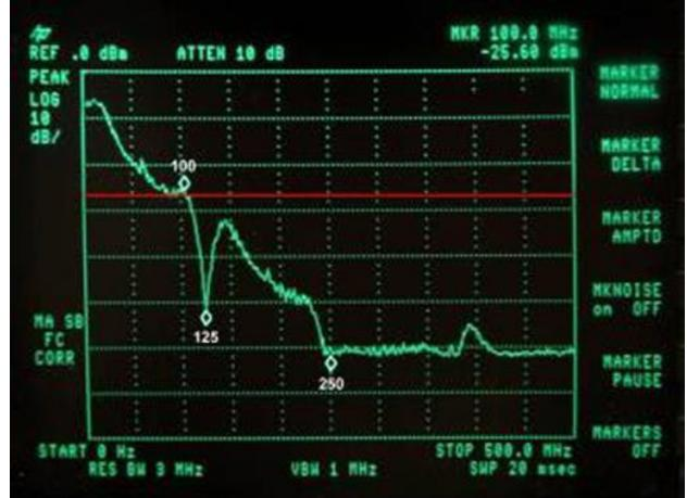
Figure 4: Frequency spectrum of 100BaseT-Ethernet
