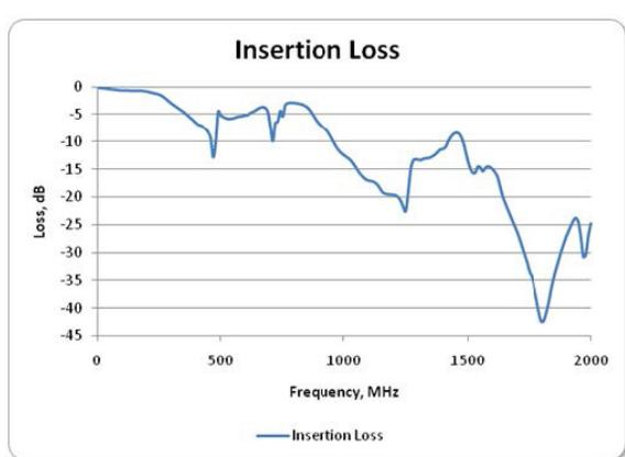
Figure 12: (0.5 Bore) Slip ring bandwidth
