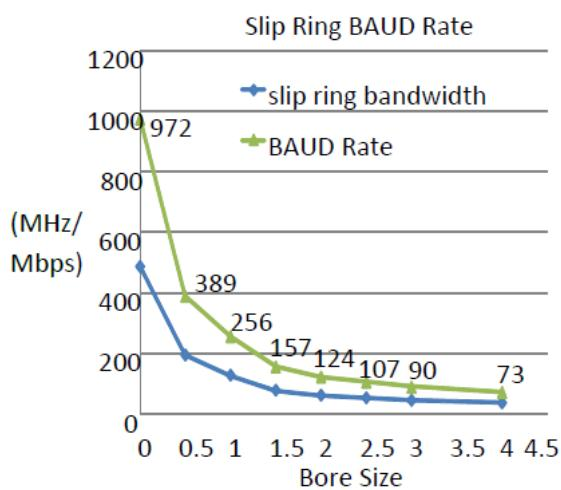
Figure 6: Bandwidth limit of slip rings as a function of bore size
