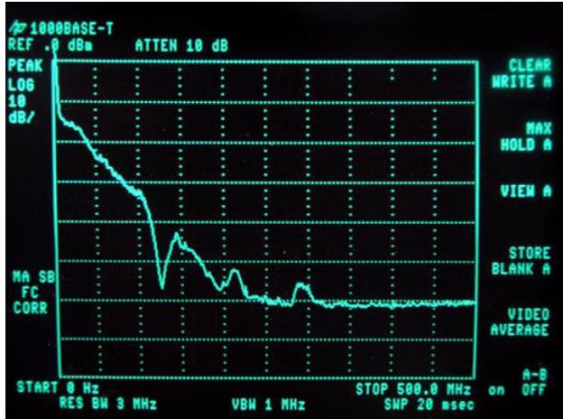
Figure 5: Frequency spectrum of gigabit ethernet (1000Base-T)
