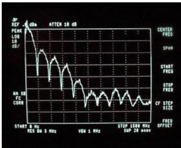
Figure 3: Frequency spectrum of 150 Mbps hotlink
