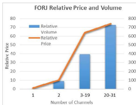
*Figure 18: This figure shows the relative difference in price and volume of multi-channel FORJs compared to a single channel FORJ (relative values of 1). These differences occur in jumps.*
