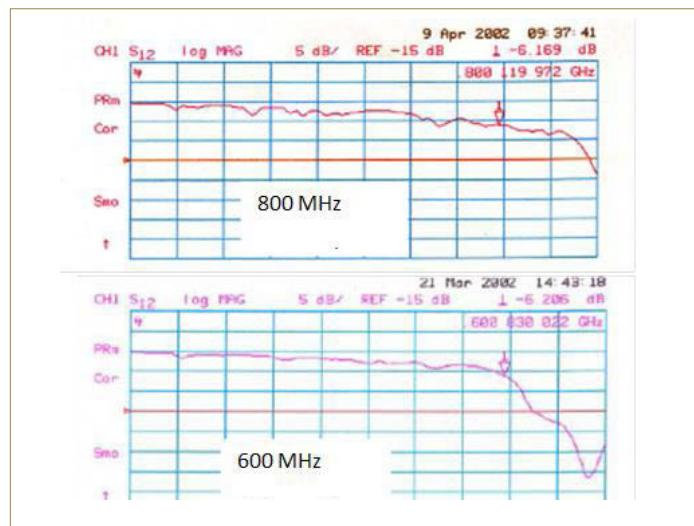
Figure 7: Insertion loss vs. frequency of two different diameter ring pairs
