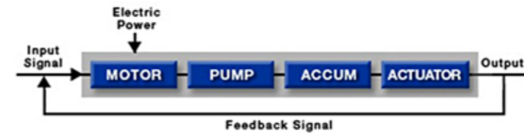
Figure: General layout of an electro-hydrostatic actuator (EHA)
